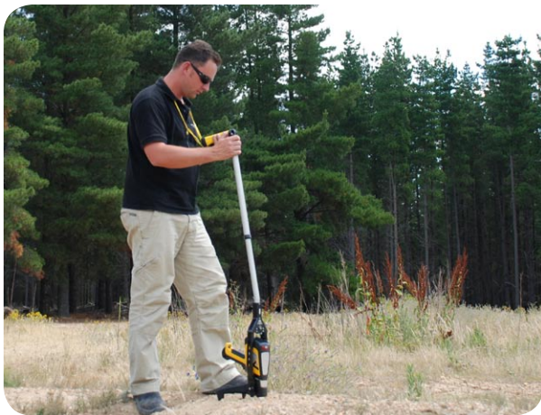
In-situ Soil Analysis with Soil Stick
