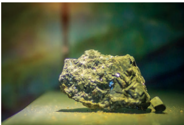
Molybdenite rock specimen from mining and quarrying industries. Molybdenite is a mineral of molybdenum disulfide, MoS 2 .
