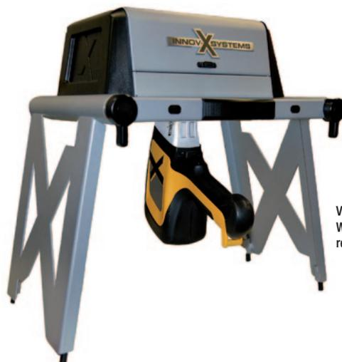
Versatility - The DELTA can be set up in its optional portable XRF Workstation, controlled by a laptop PC with full analysis and reporting capabilities.
