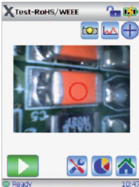
Small spot collimation for PCB component analysis
